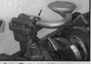
Previous ZZ engines had a 0.620-inch pickup tube and screen, but the current GM ZZ4 oil pump (PN 12555283) takes a 0.742-inch-od pickup (PN 12550042). Westech fall-safed the tube by spot-welding it to the pump body (arrow). ARP's all-steel driveshaft (PN 134-7901) spins the pump over.
