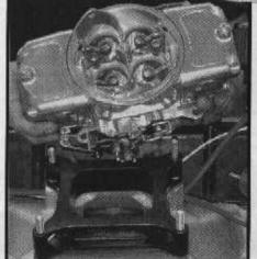
The engine ran best with a Speed Demon 850-cfm double-pumper carb on a Wilson 1-inch open spacer. Jetting was "square," with No. 92s on all four corners. A 750 proved too restrictive.
