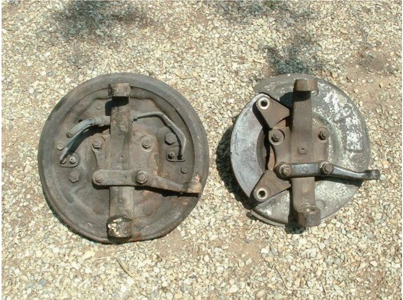
On the left: 75 Chevy LUV Factory Drum Brakes On the right: 76-80 Chevy LUV Factory Disc Brakes
